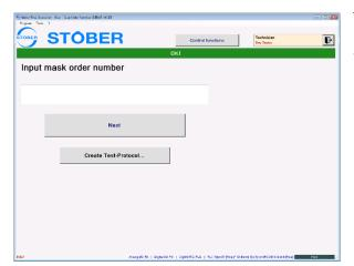
The order data can also be entered manually in an input mask in the same way as here. Usually these are loaded automatically from the system after scanning the code.
