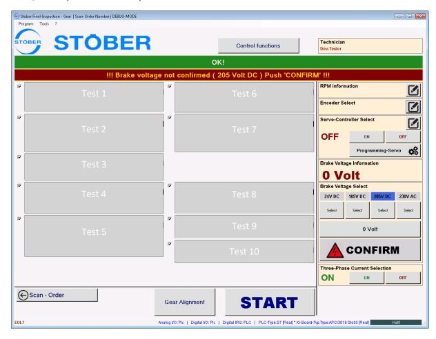
In the manual test sequence, all factors such as the target value and the tolerances can be set via the interface.
