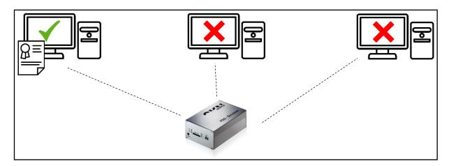
If you need several Simulyzer boxes for your measurements, you can operate several Simulyzer boxes with only one PC-ID bound license. In this case, only one software license is required to access the full functionality.
