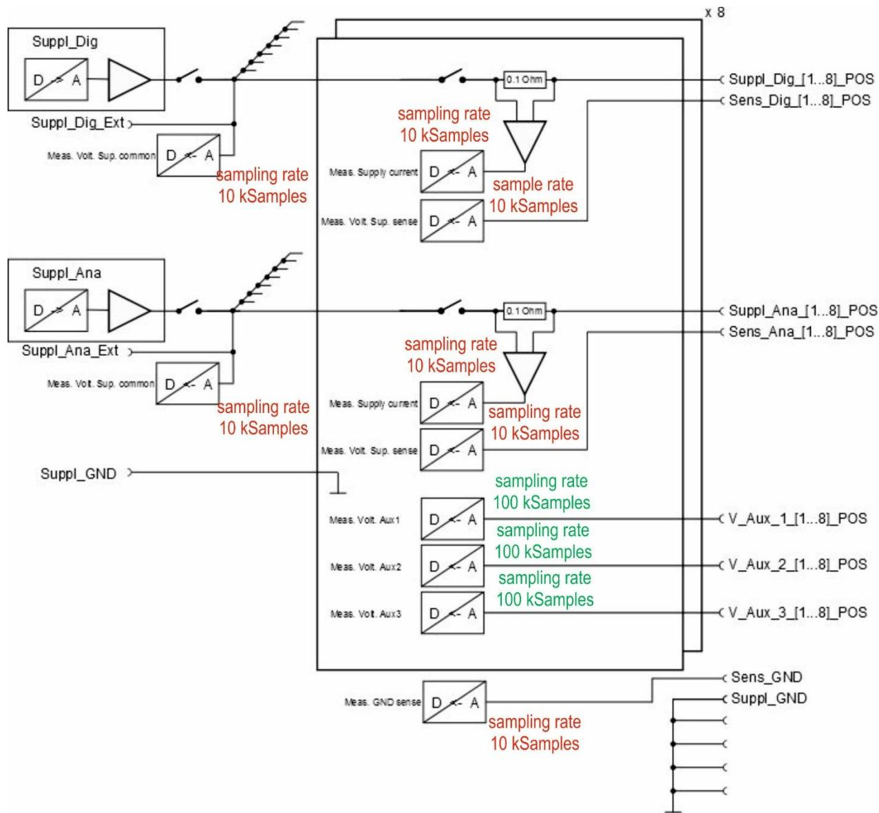
The PWR-ANA-1 card generates two turn-off voltages (Suppl\_Dig\_n und Suppl\_Ana\_n), which each supplies 2 V to 20 V/1 A. These voltages provide the 8 interfaces and can be switched on/off individually.
